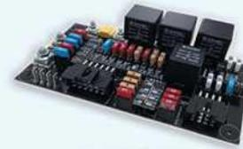
Air condition fuse & relay board
